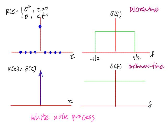
• (left) DT white noise process has a spectrum as a rectangular window
