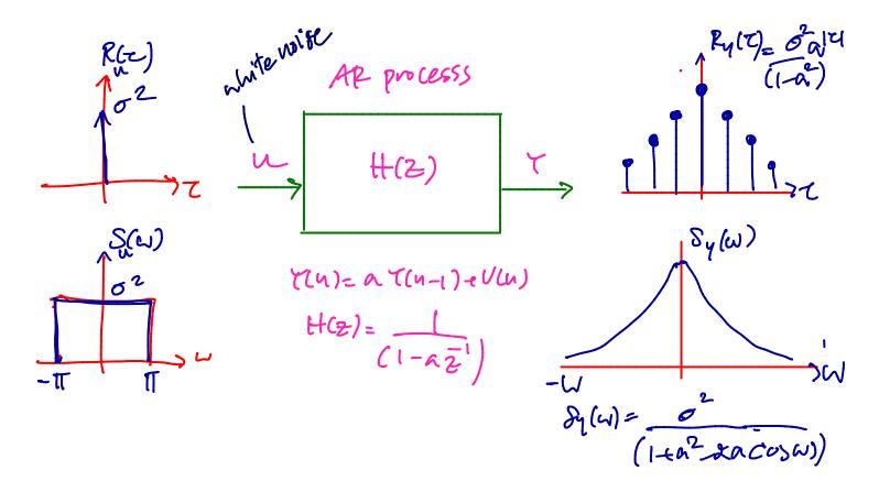
when white noise is passed through a filter, the output spectrum is no longer flat
