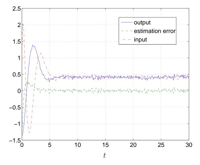
(a standard LQG does not have an integral action)
